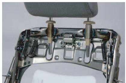
The biggest feature of this "active headrest with inertia lock mechanism" is the headrest stays at the position after moving forward at rear end collision. As the result, it obtained "GOOD" rating, which is the highest score in the whiplash injury protection evaluation test of IIHS (the Insurance Institute for Highway Safety) in USA.
