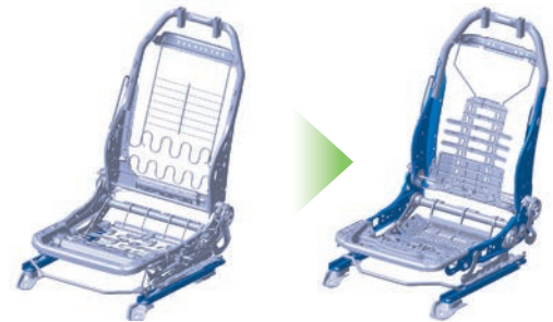
Evolution of parts using ultra-high tensile strength steel (shown in blue)
