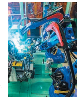
Automated welding equipment
