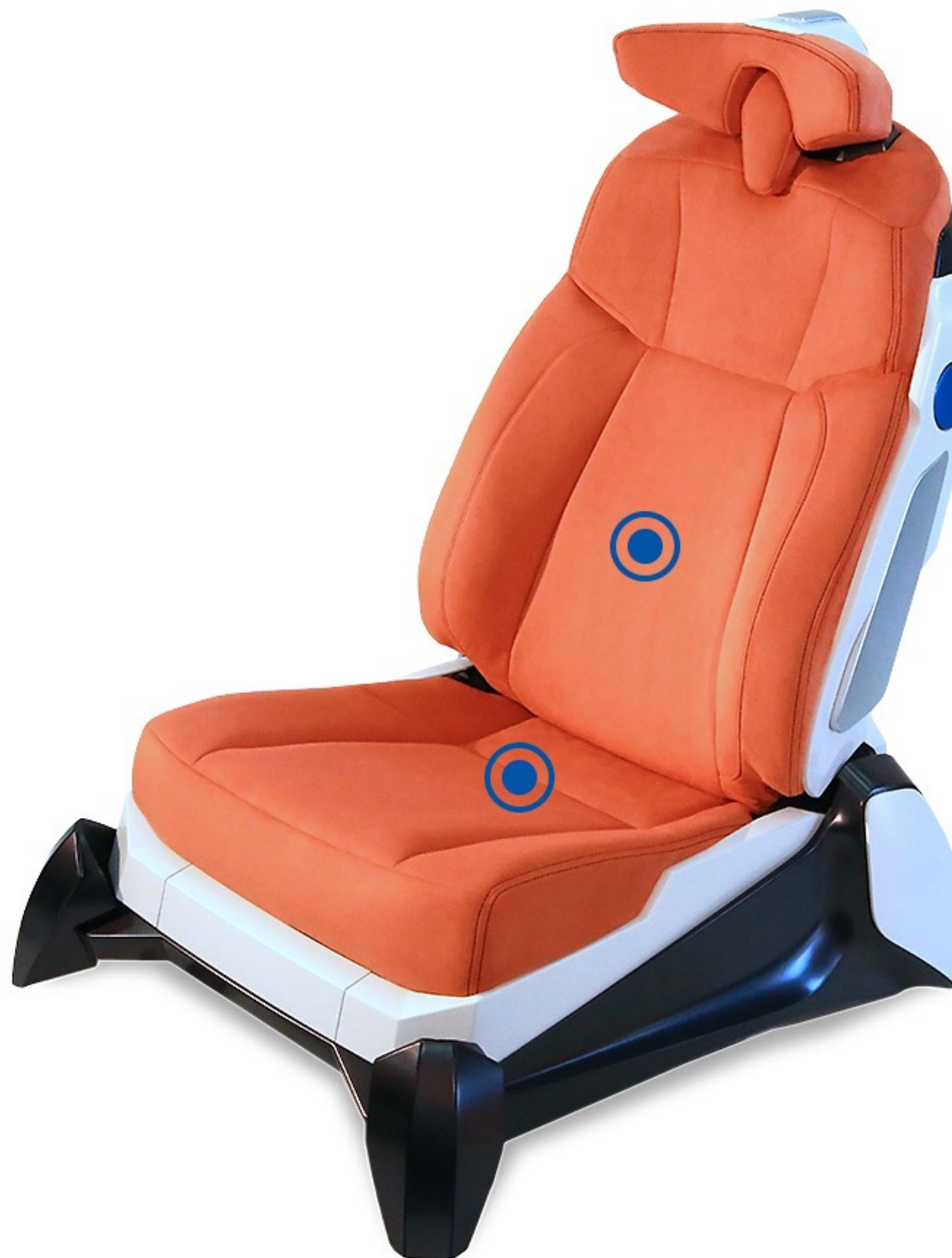
The seat measures a driver's respiratory alterations with a respiratory sensor and detects drowsiness. A vibration motor in the seatback will activate periodically to reduce drowsiness when it is detected.
