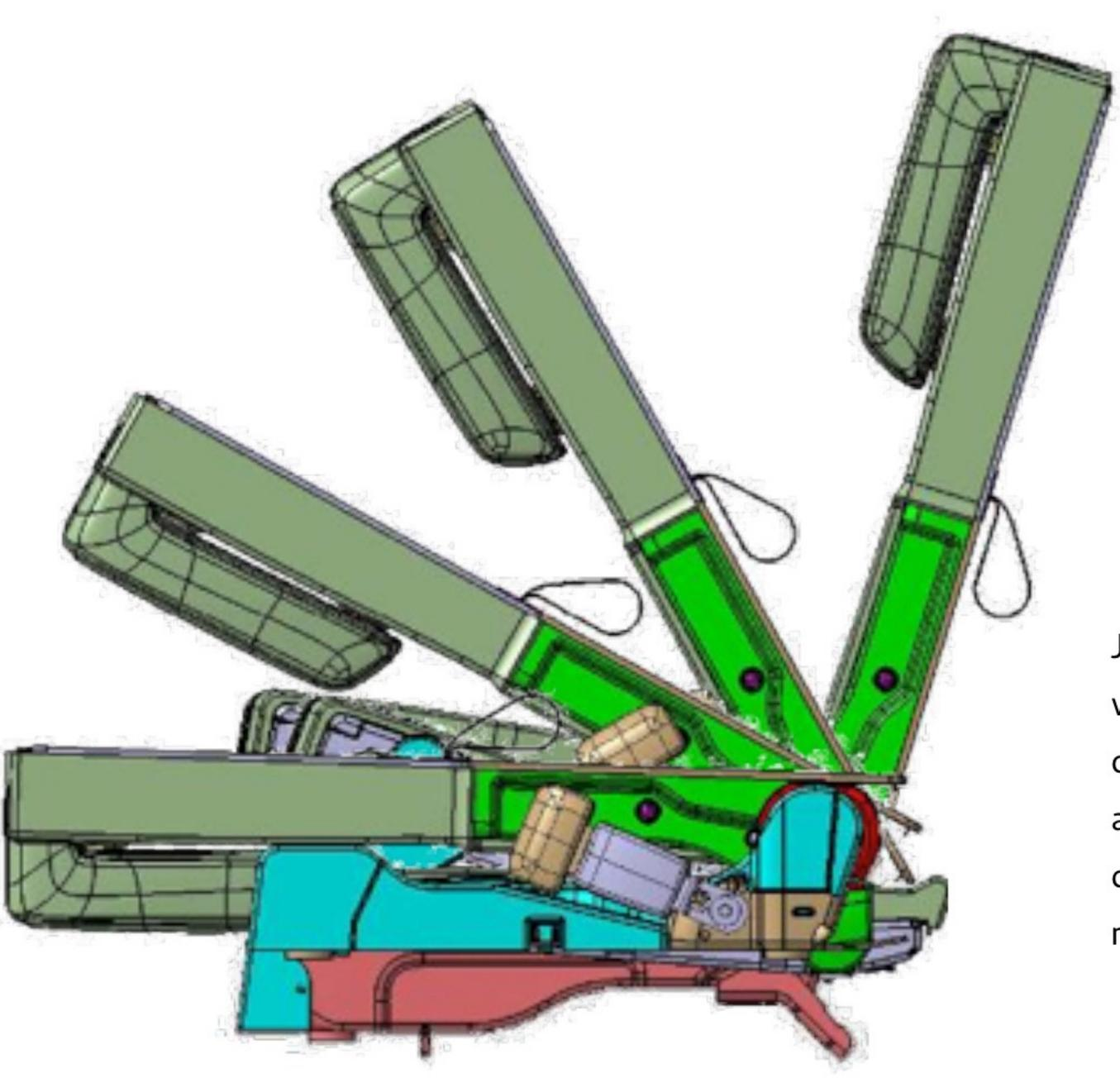
Just by pulling a knob at shoulder level with one hand, the seatback will fold down and the seat cushion will fold flat against the seatback, making it possible to create a fully flat luggage space without removing the headrests.
